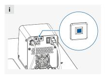
The device integrated two resetable thermal circuit breakers. They protect the device from overload conditions, e.g. too high current or too high ambient temperature.
